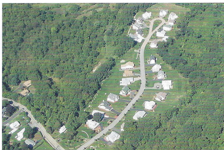
By eliminating detention pond, the subdivision layout conserves trees while 15,000 sf (1500 m 2 ) PICP in the cul-de-sac returns rainfall to the water table in Glen Brook Green subdivision in Waterford, CT.
