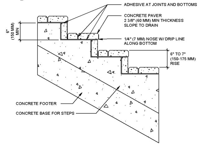
F MORTAR IS NOT RECOMMENDED EXCEPT IN NON-FREEZE-THAW AREAS. RIP LINES INTO BOTTOMS OF ALL STEP NOSES.
