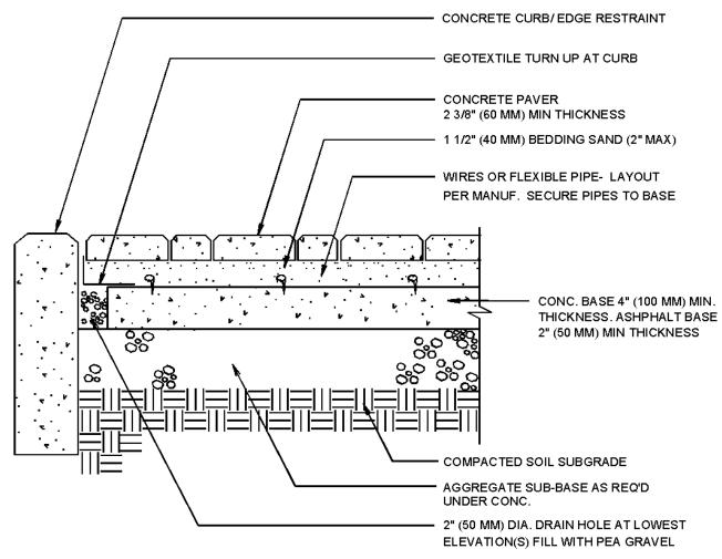
NOTE: SECURING PIPES OR WIRES TO BASE IS NOT REQUIRED FOR PEDESTRIAN APPLICATIONS
