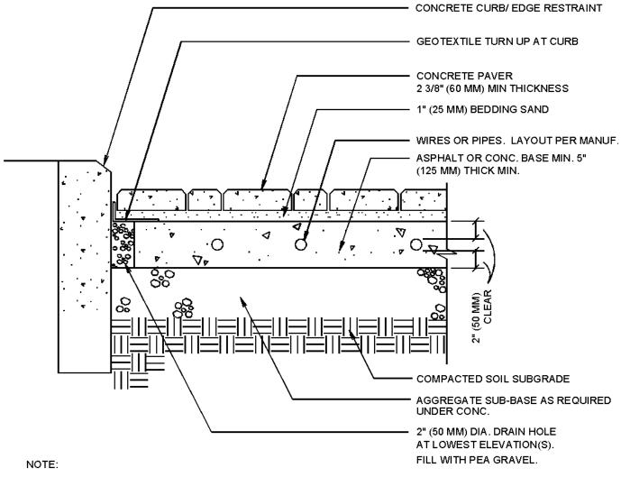
THICKNESS OF AGGREGATE BASE WILL VARY WITH SUBGRADE CONDITIONS AND CLIMATE. COLDER CLIMATES MAY REQUIRE THICKER BASES.
